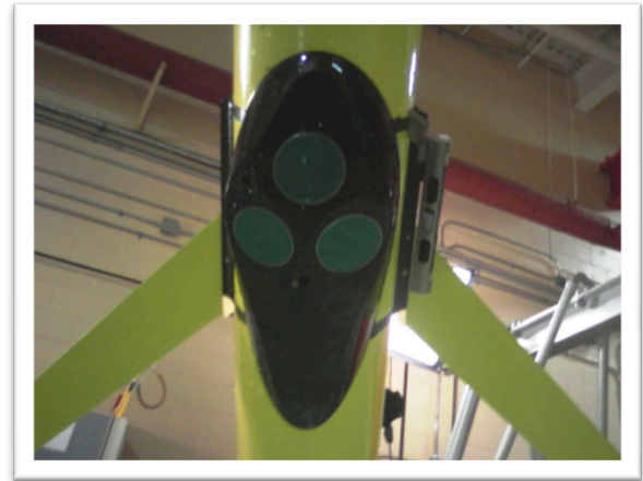
Figure 3. View of 400 kHz Nortek Aquadopp Profiler mounted on the underside of a Webb Slocum glider operated by researchers at Memorial University.
