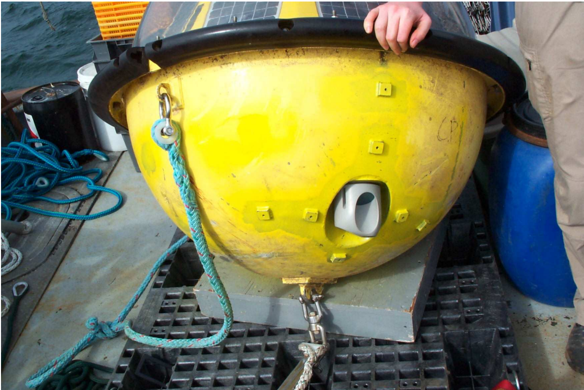
Figure 1. Nortek ACP mounted in TRIAXYS™ Directional Wave Buoy Hull
