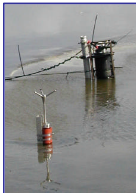
Figure 1. The Vector (foreground) and the ADVO were deployed 2 m apart and measured velocity at an elevation of about 0.5 m above the sand.
