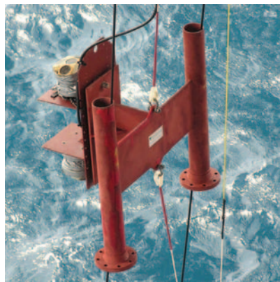
Figure 2. Platform Mount AWAC being lowered into place on oil platform. Downward looking AWAC is used for current profile measurements into deeper water. Photo: B. Magnell, Woods Hole Group
