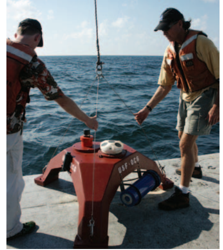
Figure 5. AWAC being deployed on a bottom frame in the Gulf of Mexico. Real-time wave data are processed by NIP and sent to the surface buoy via underwater acoustic modems.
