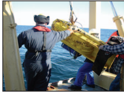
Figure 4. AWAC being deployed on subsurface buoy at offshore location for site survey. Photo: J. Barthelotte, Bedford Institute of Oceanography.
