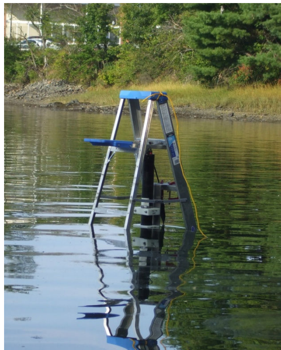
Figure 1 – Eddy-correlation device deployed in Kittery, Maine
