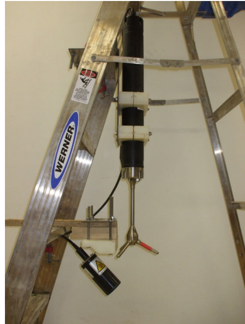
Figure 2 – Nortek Vector ADV (A) and WETLabs CDOM fluorometer (B) mounted on ladder.
