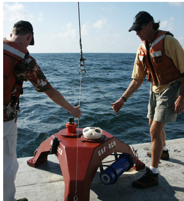
AWAC equipped with an external battery canister and underwater acoustic modem being deployed in the Gulf of Mexico.
