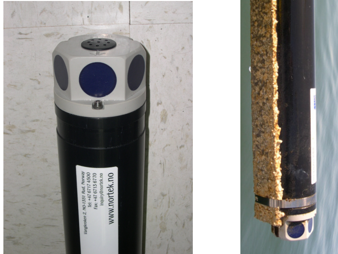
Figure 2. ASCM with 3 horizontal transducers and mounted on bracket with transducer head 1.0 m below the surface. A pressure sensor is housed below the black plastic cover on the top of the transducer head. A cable connects from the end-cap of the ASCM to the real-time telemetry system on the NOMAD buoy.
