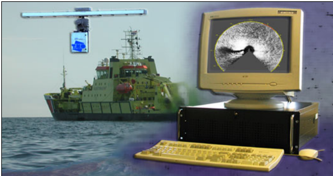
Figure 1: HH/VV antenna, Xband radar; ship (The Arca, The Netherlands) with SeaDarQ system installed, and displaying an oil spill image.
