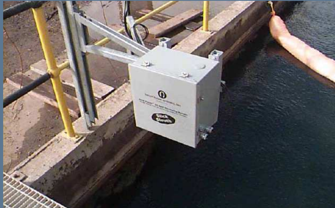
UV fluorosensor SlickSleuth, source InterOcean Systems
