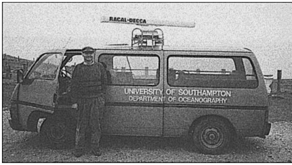
FIG. 1. Photograph of marine radar deployed from a van at a coastal location.
