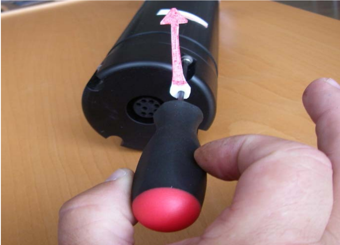
«Two-finger» tightning of screws. Indicator arrow shows position before final tightning
