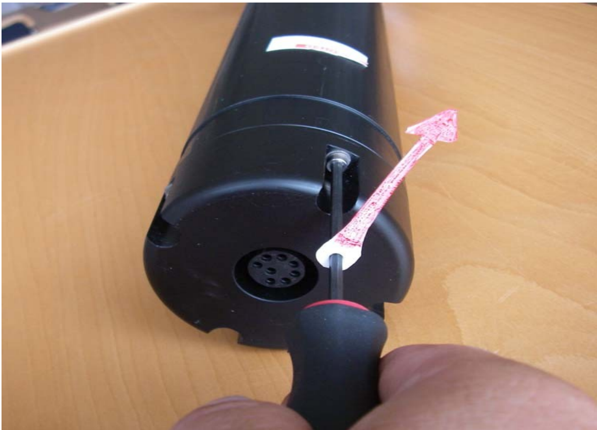
Final tightning 30-45 degrees from «two-fingers» tightning
