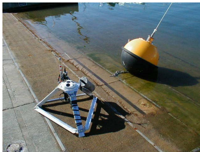
Fig. 5 Waverider and AWAC (center of triangular frame) prior to deployment, Carqueiranne, France.
