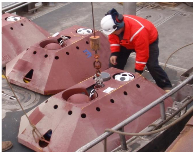
Fig.2 Three Nortek AWAC's in fiberglass bottom frames with acoustic pop-up floats were deployed in the Beaufort Sea for one year.
