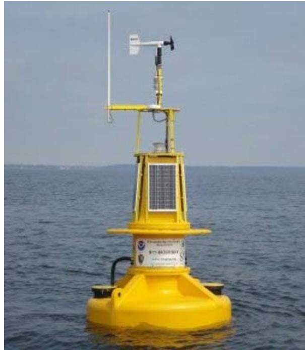
Fig. 1 Buoy with AXYS Technologies TRIAXYS directional wave sensor and a downward looking 1 MHz Nortek Aquadopp Profiler.
