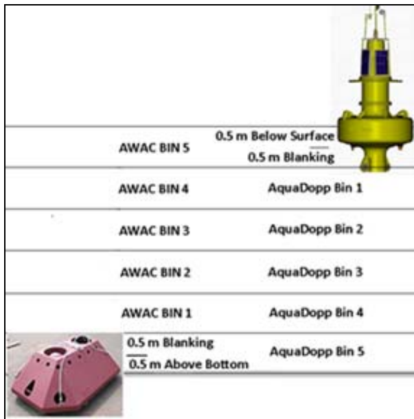
Figure 2. Relative locations in the vertical of AWAC and buoy AquaDopp velocity bins.
