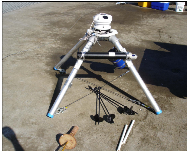
Fig. 1. The AWAC was mounted on the top of the Nortek Aquaquad Deployment Frame and fixed to the bottom utilizing fence anchors.
