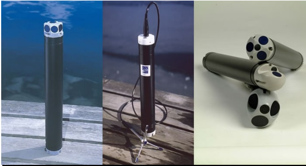
Figure 5 Nortek instruments that measure waves using the PUV method. From left to right (a) Aquadopp, (b) Vector, (c) Aquadopp Profiler.
